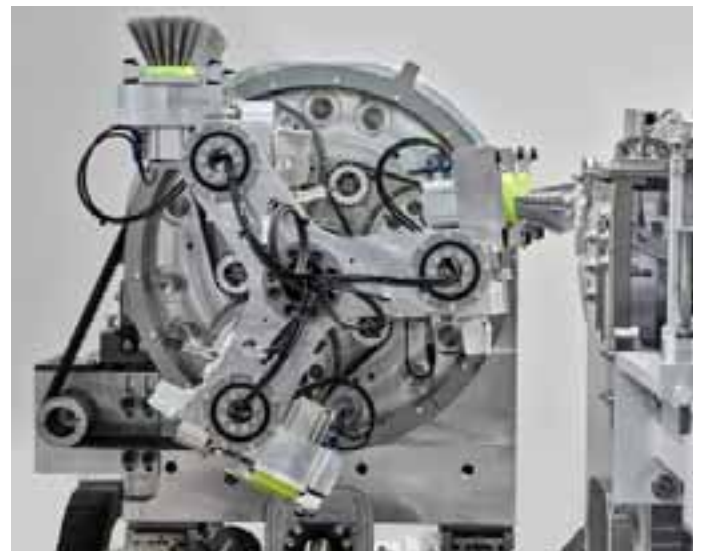
NM is laid out as a small carousel with just 3 clamping stations. Loading happens far away from tool and drill.
