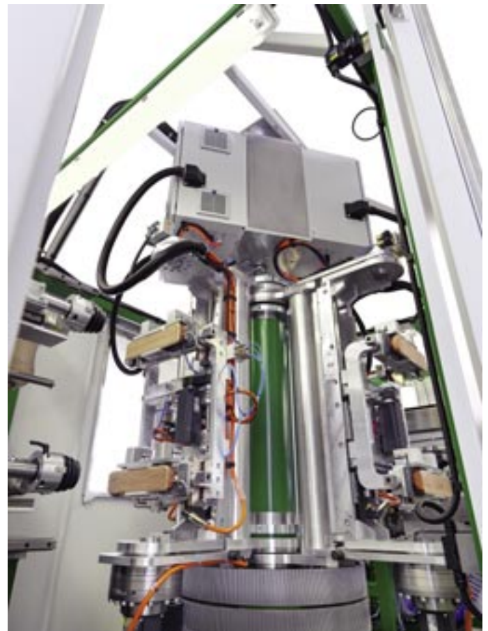
Five-station carousel with "Roth flying cabinet" (Photo: Roth Composite Machinery)
